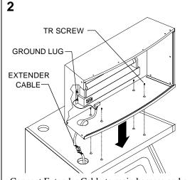
Connect Extender Cable to main harness and run it through holes in top of cabinet and bottom of Header Housing. Connect it to Lamp Assembly. Place ground lug over bottom left stud on Lamp Assembly and fasten with ESN nut. Align Housing with holes atop cabinet and fasten with tamper resistant screws.
